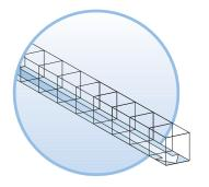
**Level fall** A straight channel run, when no fall is needed or the natural fall suffices.
